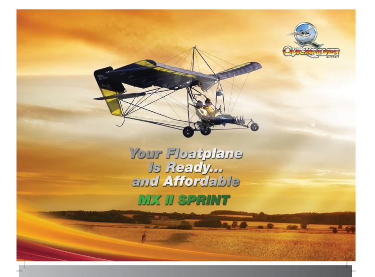
THE MX II SPRINT'S HIGH LIFT, PARTIAL DOUBLE SURFACED WING GIVES IT AN EXCEPTIONALLY SHORT TAKE OFF ROLL AND PREDICTABLE HANDLING AT VERY LOW FLIGHT SPEEDS.
